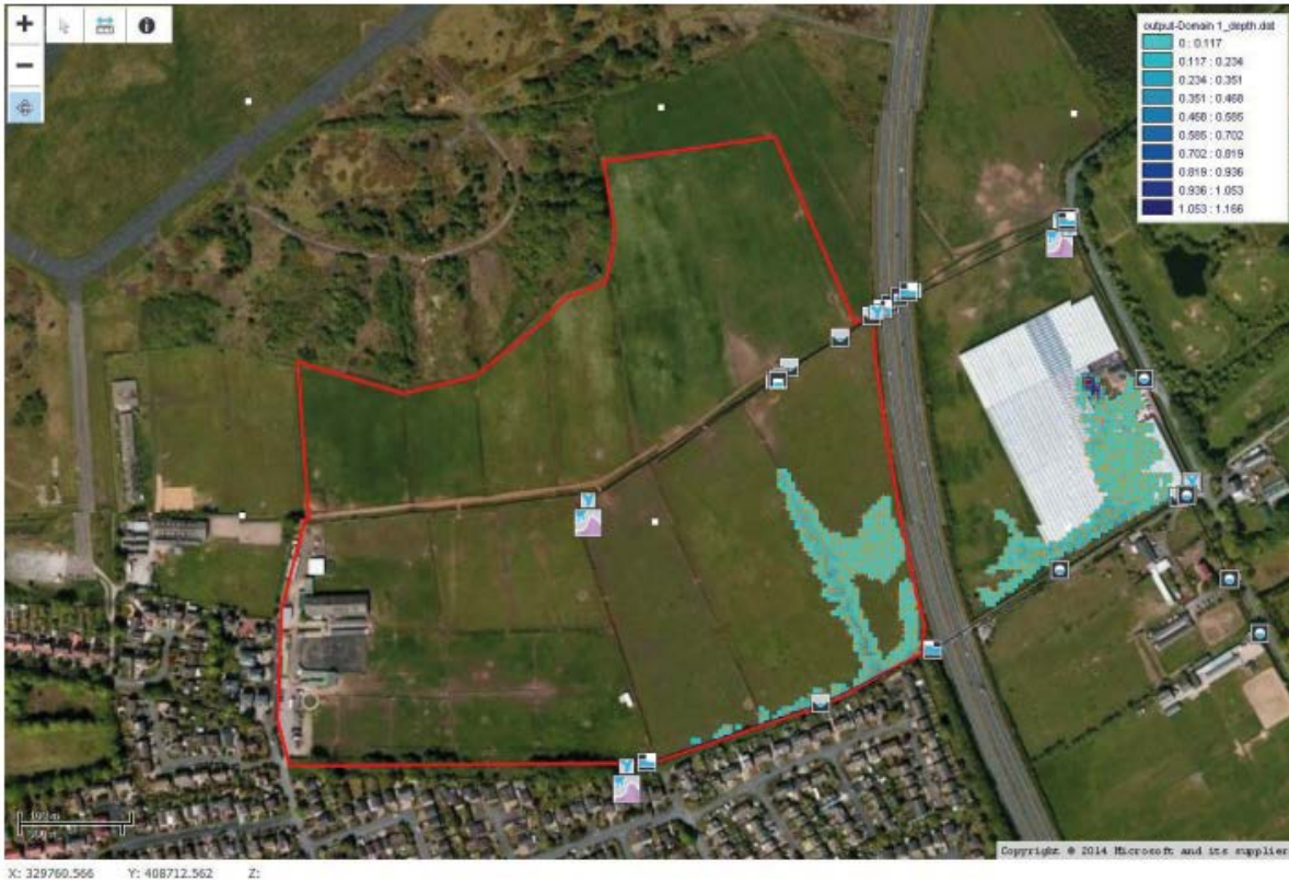
Figure 7.3 -Pre Development Flood Model (detailed topographical survey)
